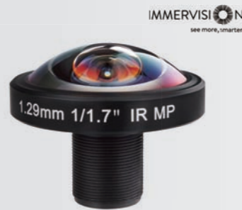
Model No. (型号) E3279A φ5.4mm f1.29mm FOV190° F-theta distortion: +25.5%
